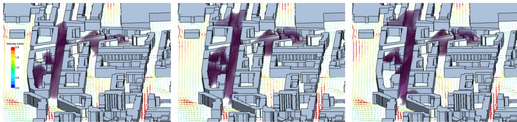
**Figure 5.** Dispersion of NO<sub>x</sub> passive scalar at (left) 5 min, (middle) 15 min, and (right) 30 min following spin-up from the prototype run. Mean wind travels from the bottom to the top of the figures.
