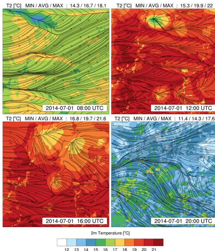
**Figure 2.** Two-meter temperature (contours) and ten-meter horizontal wind (streamlines) of nested WRF domain (horizontal resolution 500 m) at 8:00, 12:00, 16:00 and 20:00 UTC on July 1<sup>st</sup>, 2014. The city of Berlin is located roughly at the center of the domain.
