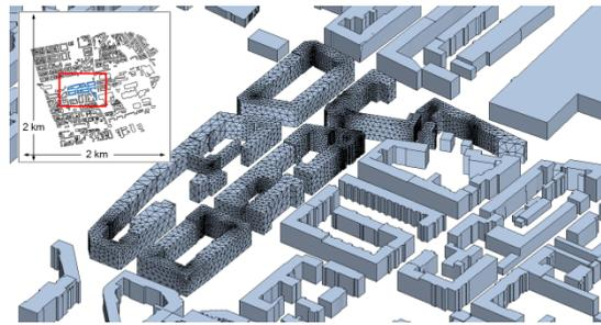
**Figure 4.** Close-up of the prototype run with region of interest highlighted (tessellated). Inset indicates horizontal extent ( $2 \text{ km} \times 2 \text{ km}$ ) of the urban model domain.
